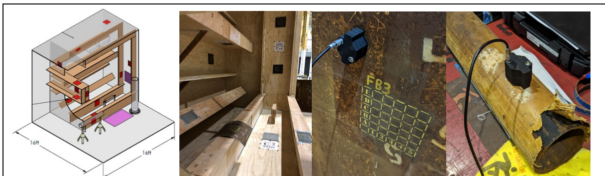
Figure 1: Pictures left to right: illustration of FPSO hull mock up showing red locations of test samples with thicknesses unknown to the inspector, picture of actual FPSO mock up structure (wooden structure with changeable steel test samples), EMAT probe on steel sample and EMAT probe on pipe sample.
